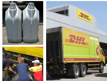
Photos: for benchmarking purposes, A/C fuel lines were disconnected from main fuel tanks and plugged into 5L bottles.
