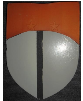
Above: painted clay roof tile. Left side: Planet Supra Right side: Planet Supra Neo
