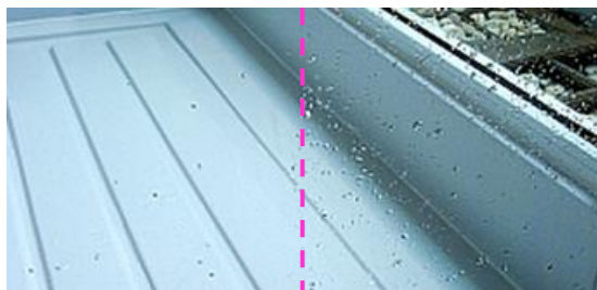
Glass shower door: the coated left side is almost free of droplets, the right side is not sealed.
